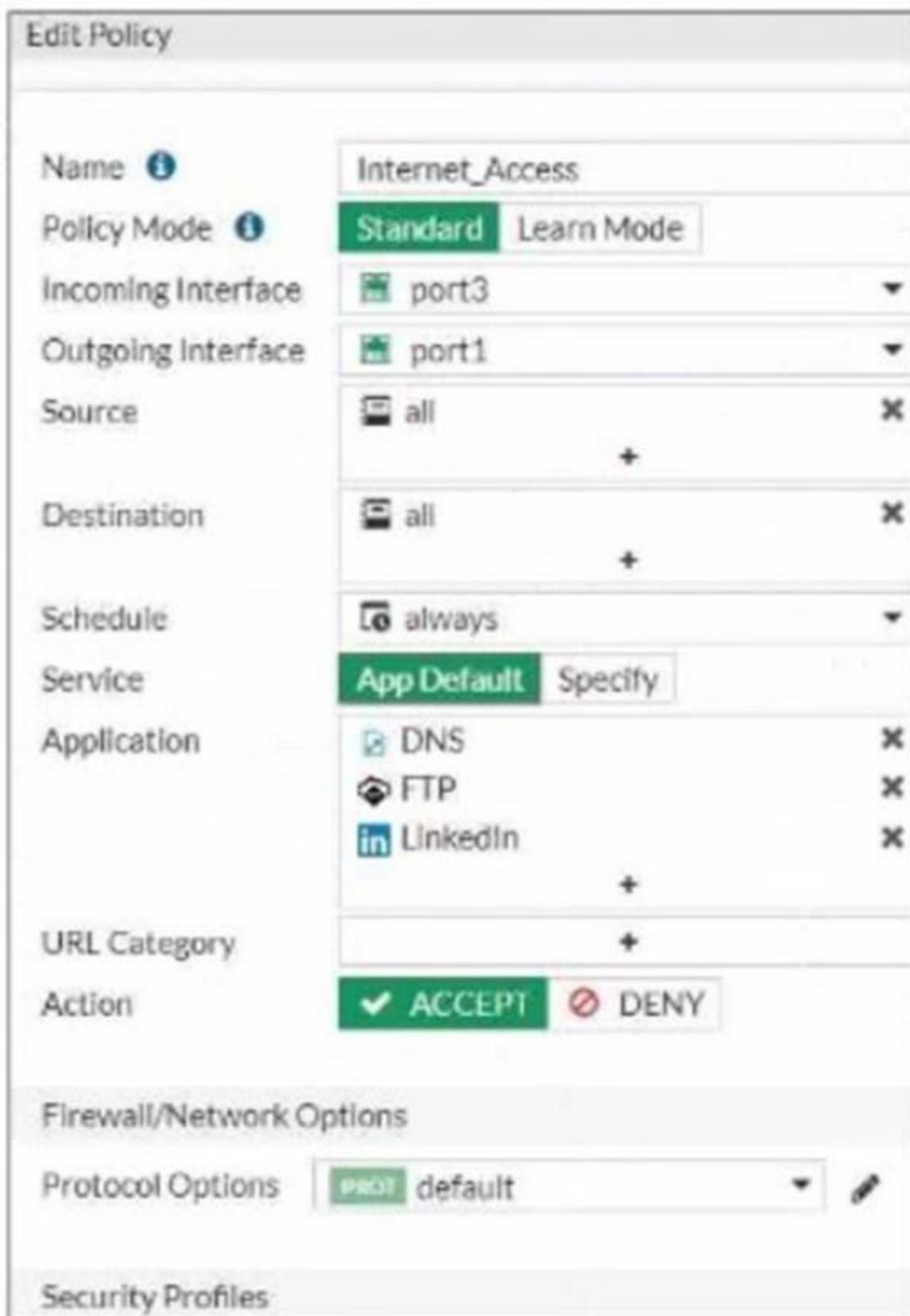
Refer to the exhibit, which contains a partial policy configuration. Which setting must you configure to allow SSH?
