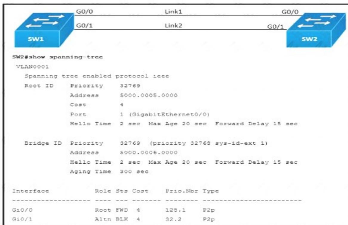
Link1 is a copper connection and Link2 is a fiber connection. The fiber port must be the primary port for all forwarding. The output of the show spanning-tree command on SW2 shows that the fiber port is blocked by spanning tree. An engineer enters the spanning-tree port-priority 32 command on GO/1 on SW2, but the port remains blocked. Which command should be entered on the ports that are connected to Link2 to resolve the issue?
