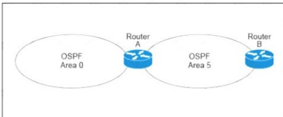
A customer runs OSPF with Area 5 between its aggregation router and an internal router. When a network change occurs in the backbone, Area 5 starts having connectivity issues due to the SPF algorithm recalculating an abnormal number of times in Area 5. You are tasked to redesign this network to increase resiliency on the customer network with the caveat that Router B does not support the stub area. How can you accomplish this task\*?
