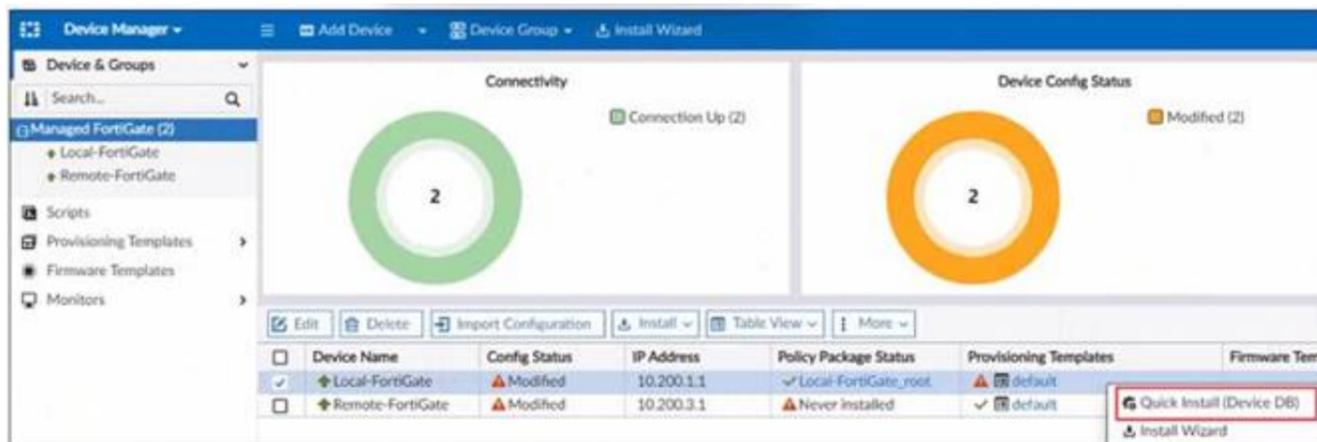
You are using the Quick install option to install configuration changes on the managed FortiGate
