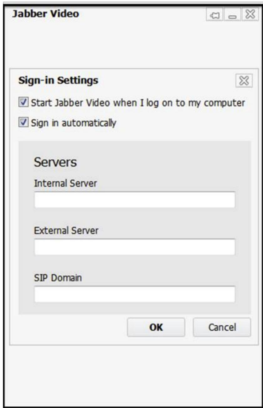
When the Cisco Jabber Video for TelePresence fails to register with the server, which two fields should be configured at a minimum, assuming SRV records are not configured? (Choose two.)
