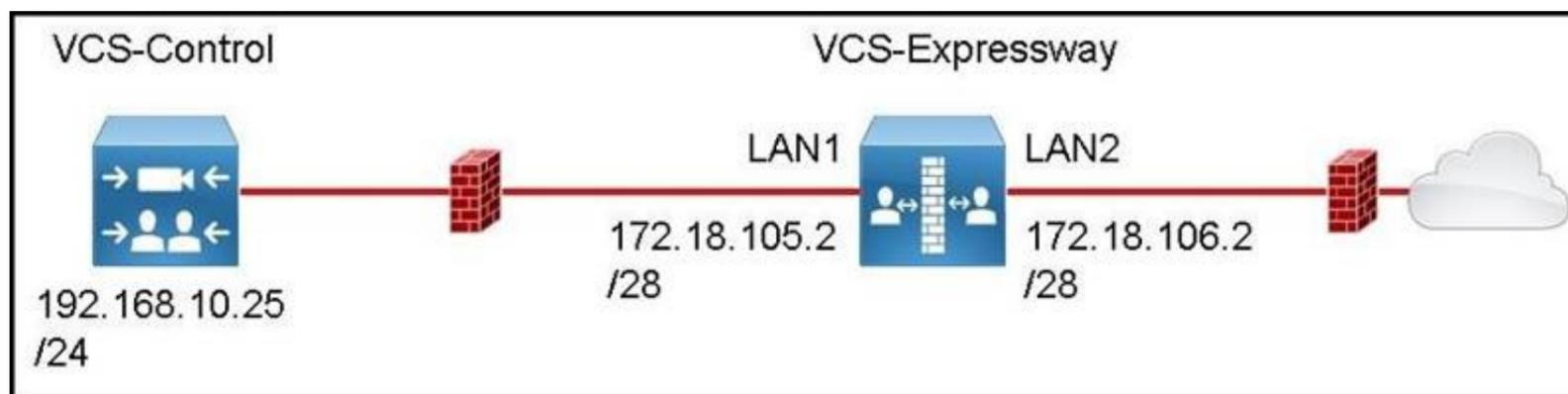
You are deploying a Cisco VCS Expressway with the Advanced Networking option key into two separate DMZs. Gateways for all networks are the lowest usable IP address in the subnet. While you are logged in as an admin user, which command should you enter into the CLI, to enable IP routing to the Cisco VCS Control and nothing else on the internal network?
