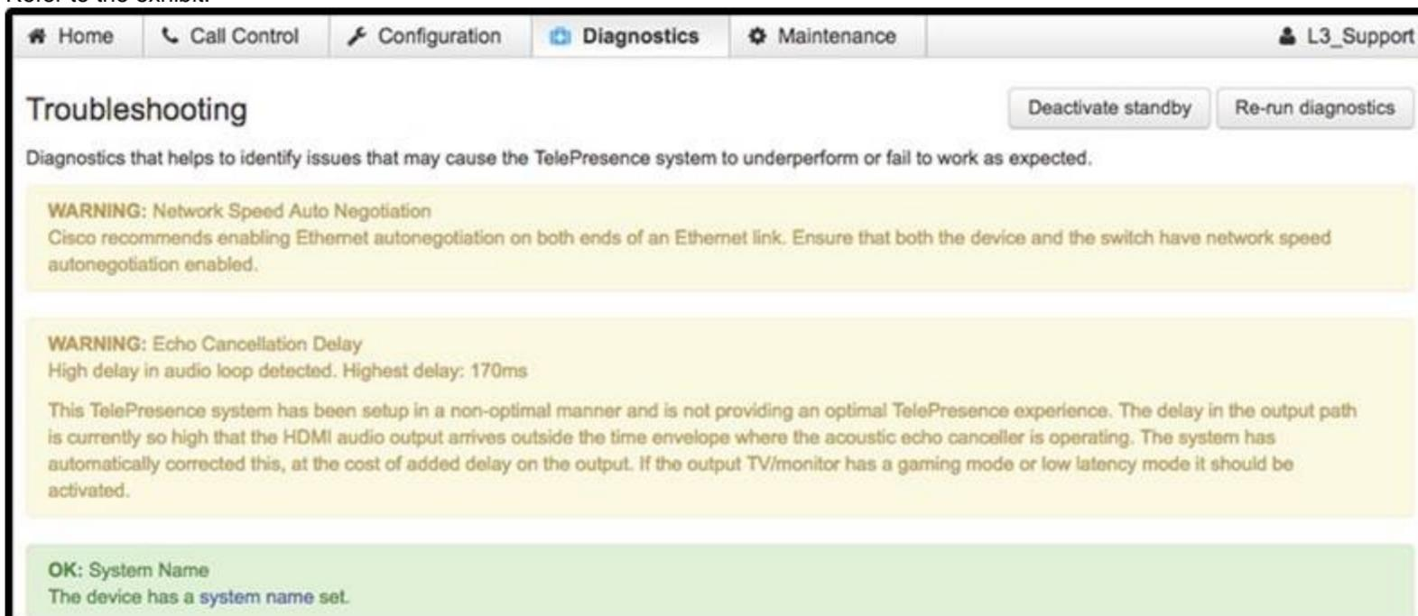
The customer recently connected a new TV monitor to the Cisco TelePresence endpoint. This device is now showing a warning concerning the echo cancellation delay. Which action could help mitigate this issue?
