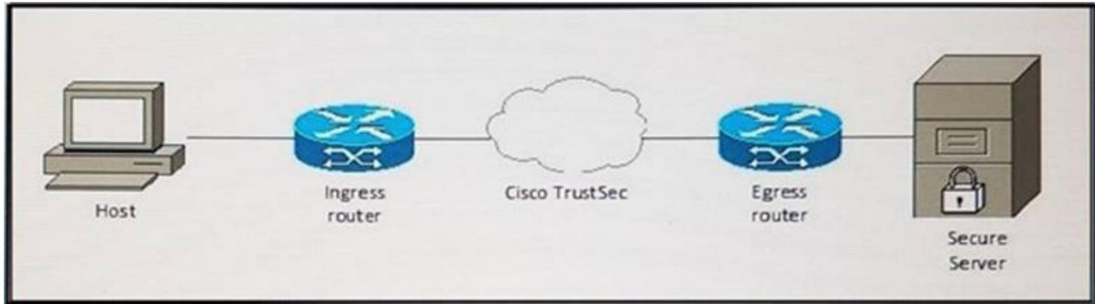
If the host sends a packet across the Cisco TrustSec domain, where is the SGACL enforced?
