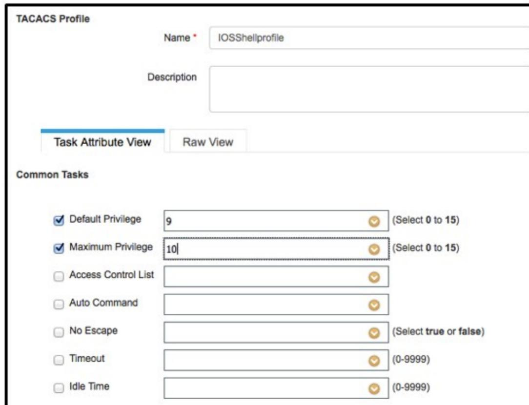
The screenshot shows the configuration for a TACACS profile named 'IOSShellprofile'. Under the 'Common Tasks' section, the following settings are visible:
