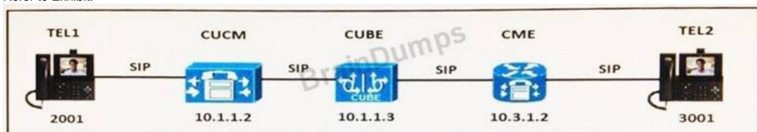
An engineer is working on a ticket that reports TEL1 cannot call TEL2. These dial peers are configured to route the call between the endpoints.
