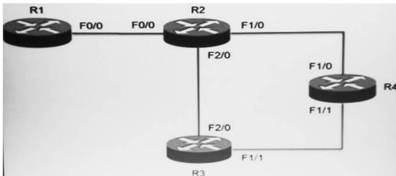
MPLS TE Tunnel 138 has a headend R1 and a tailend R4, and uses path R1-R2-R4 as the primary LSP. The path R1-R2-R3-R4 should be implemented as a backup LSP in case the R2-R4 link fails. To which interface should the appropriate configuration be applied to accomplish this?
