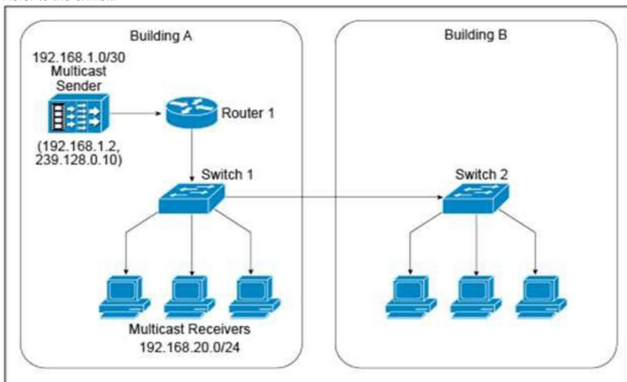
A new IPv4 multicast-based video-streaming service is being provisioned. During the design- validation tests, you realize that the link between the two buildings is carrying multicast traffic even when there are no receivers connected to the switch in Building B and despite IGMP snooping being enabled on both Layer 2 switches and IGMPv2 runs on the hosts. Which design change will prevent the multicast traffic from being unnecessarily flooded throughout the campus network?
