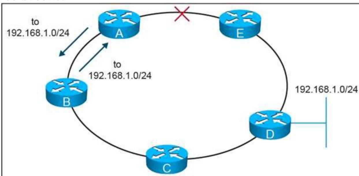
On this MPLS-based network ring, links have failed between router A and router E. These failures formed microloops while the network converged, when A forwarded traffic to B but B forwards it back to
