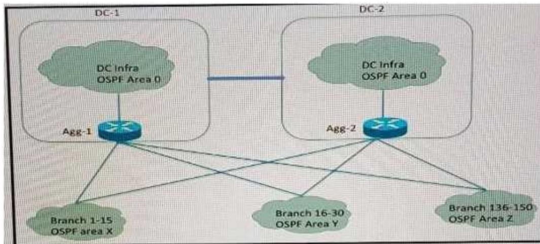
company xyz has 150 branch location across the U.S. Each branch is connected to two aggregation router one router in each data center The network is configured with Multiple OSPF with multiple OSPF areas and the aggregation router are ABRs A requirement is to keep an optimal path to the data centers and at the same time reduce the LSA propagation and SPF recomputation during a change in any part of the network Which design elements should be included on the aggregation router?
