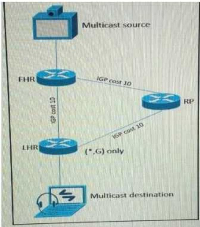
As part of a redesign project, you must predict multicast behavior. What is the resultant multicast traffic receiving on the shared tree( , G), if it is received on the LHR interface indicated?
