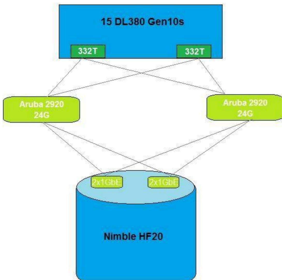
A customer purchased a server/storage environment shown in the exhibit with 1 Gb networking connectivity. The customer is now experiencing performance issues. Identify the correct components to upgrade the network connections and improve performance on the left. Then drag those components to the answer area on the right. (Choose three.)
